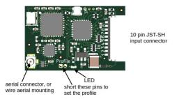
MT01b does not have an on-board LED. You will need to connect JST-SH 6p, pin 3 to an external LED - see one of the wiring diagrams below for an example LED connection.
