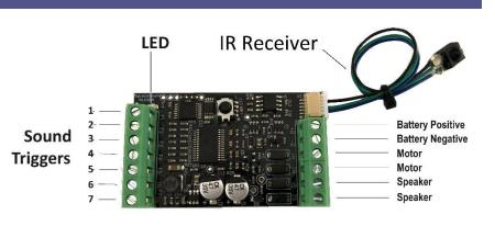
the vehicle controller has the appropriate outputs available. The trigger terminals are labelled F1 to F7 and are referred to by these labels in these instructions. For example, "Triggering F1" means to close a contact between the F1 terminal and the Battery negative terminal.
